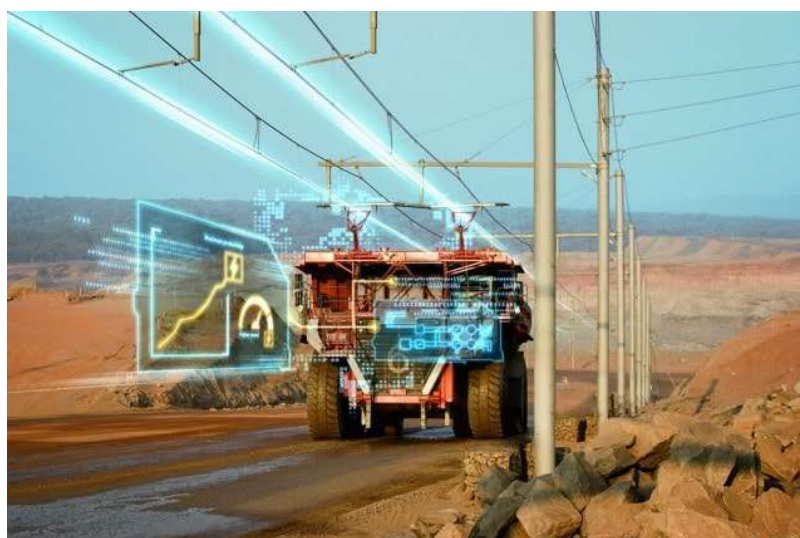
Figure 10: Trolley system for heavy mine hauling trucks in Australia (Source: https://www.australianmining.com.au/mining-decarbonisation-innovations-charge-on/ ).
