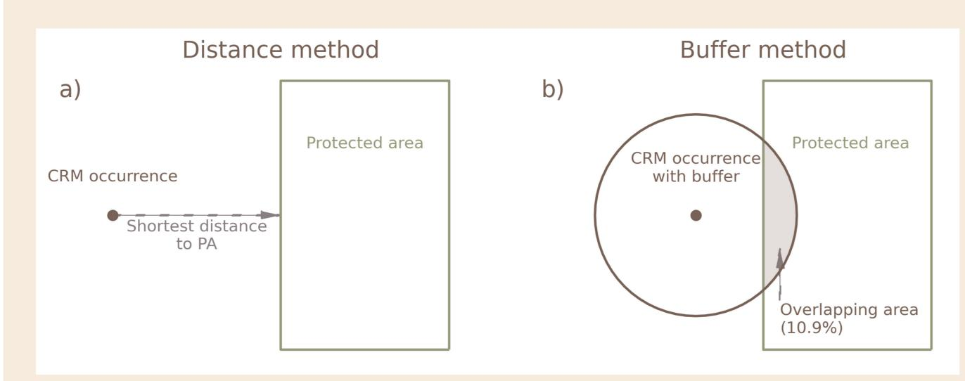
Illustration of the a) distance and b) buffer method for analyzing overlap of CRM occurrences with PAs. The proportion of CRM buffer area overlapping with the PA is 10.9 %.
